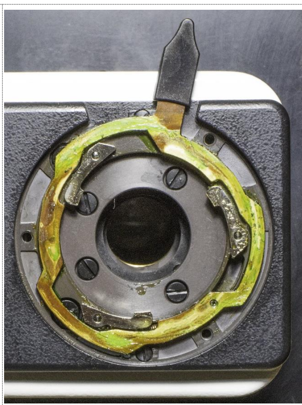
Figure 5: View down on the head mount, collar removed, showing the head release mechanism (lever and three metal clamps).
