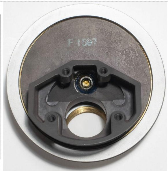
Figure 9: The nosepiece, view from the top.
