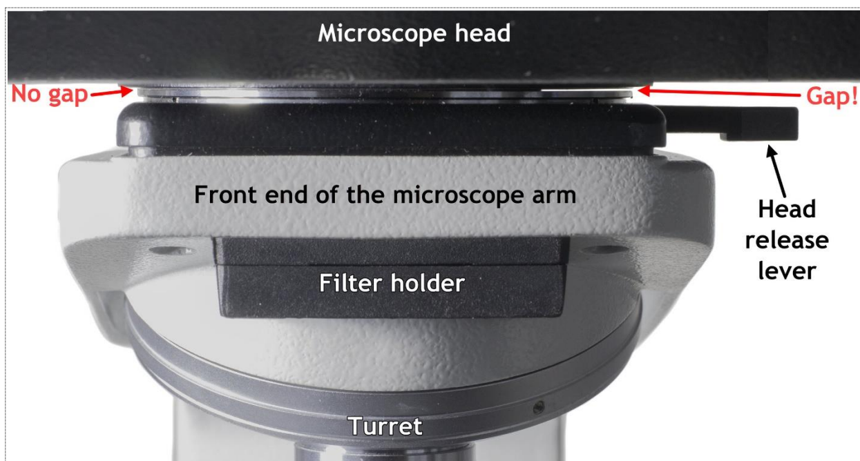
Figure 18: A small gap between the underside of the head and the collar of the microscope's head mount reveals that the head is not properly attached to the microscope. The head in this image is slightly tilted in the microscope's optical path.
