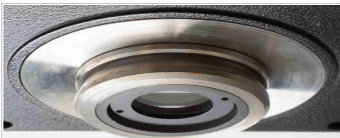
Figure 3: Dovetail mount on the underside of the head.
