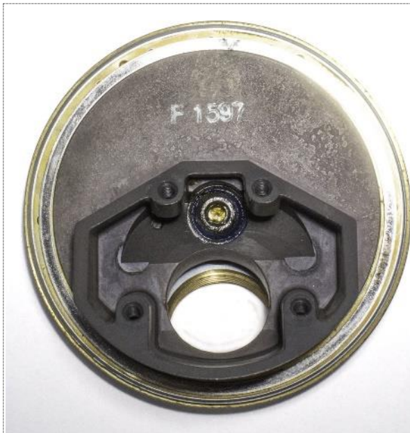
Figure 12: The nosepiece, after the threaded turret locking ring has been removed. The large turret ball bearing is now visible. The bearing balls are not visible because they are below the ball bearing race.
