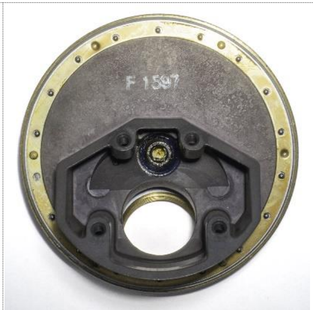
Figure 13: The nosepiece after the threaded turret locking ring and the bearing race have been removed. The bearing retainer (made of brass) and the bearing balls are now visible.
